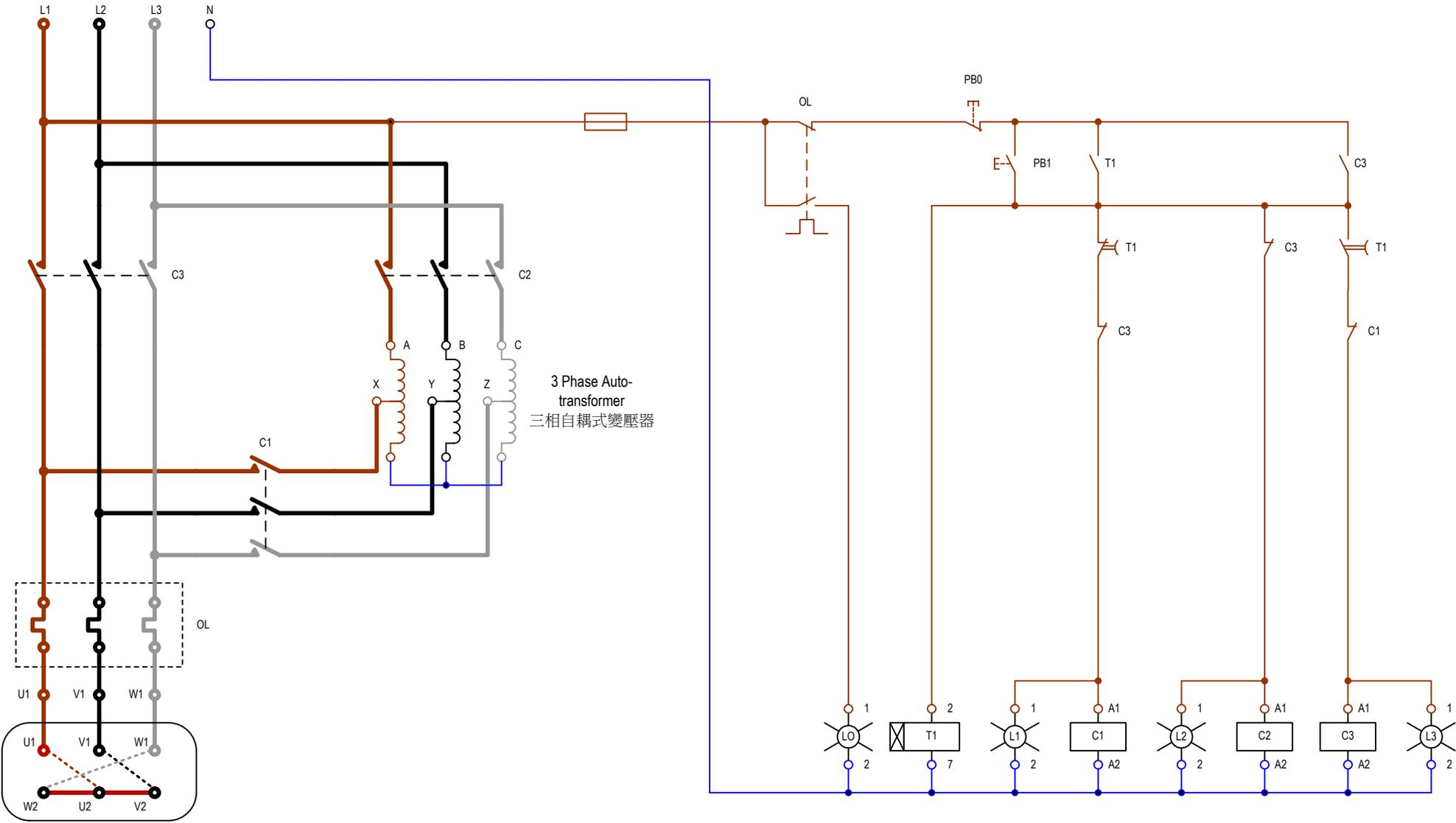
3 Phase Motor Auto-transformer Starter Circuit
